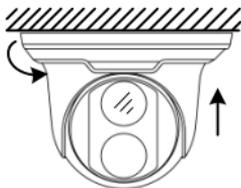
Push bottom ring back up and turn it clockwise to lock into position
