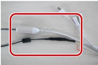
3. Protect other cables using insulating tapes.
