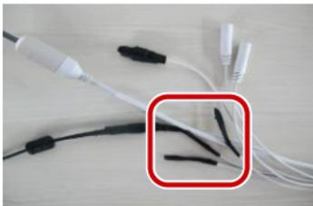
4. Wrap all the tail cables together using insulating tapes.
